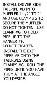
NOW GO BACK AND TIGHTEN ALL CLAMPS, NUTS AND BOLTS STARTING FROM THE FRONT AND WORKING BACK. INSTALL STAINLESS TIPS. USE ZIP TES FOR BRAKE LINES, WIRES, ETC.
